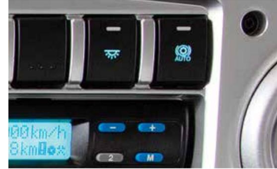
Supporting efficient use of the engine brake and the Intarder, the Smart Brake Management System, which can be activated by using the button on the front panel, makes best use of the auxiliary brakes based on braking requirements and ensures that service brakes are always ready for emergencies.
