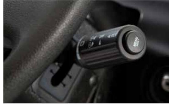
The 600 kW Intarder, which is available as an optional feature on 420 PS vehicles, meets all expectations under such challenging conditions as going downhill while loaded. Preventing unnecessary use of your service brake, it prolongs service life.
