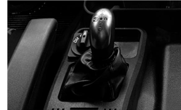
12-speed automated transmission is provided as an option for 420 PS vehicles. The system automatically selects the most appropriate gear for each situation and provides great comfort.
