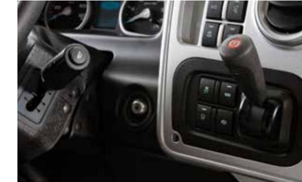
Eco, Off-Road and Rocking modes are compatible with all types of road and terrain. Eco mode provides fuel economy without compromising performance. Off-Road mode is ideal for rough terrain with its excellent traction. And Rocking mode is a powerful support against the risk of getting stuck in muddy terrain.
